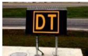
Taxiway Location Signs
