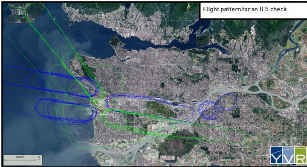
Figure 1: Sample Flight Tracks Associated with an ILS Flight Check
